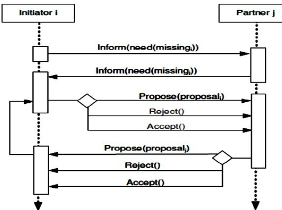
Figure 3. UML specification of the bargaining protocol..
