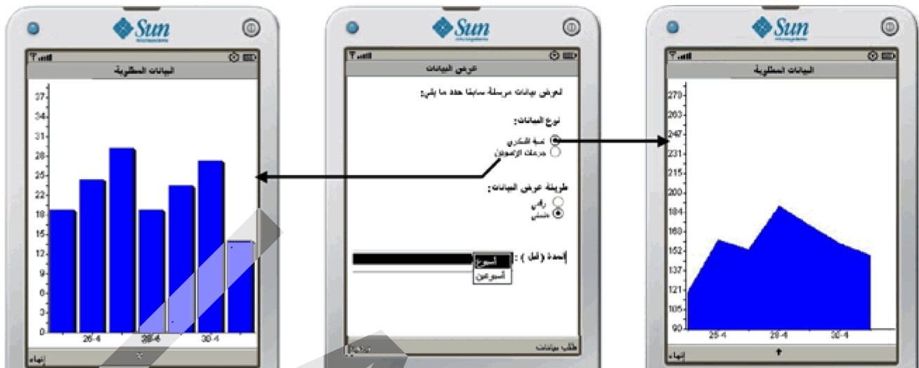
Figure 2. The patient is presented with options to select type of data to display, its form and period (center); insulin intake histogram sample (left); blood glucose measurement curve sample (right)
