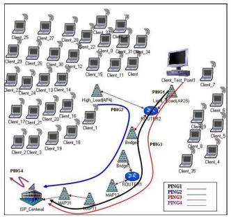
Figure (6). Network Setup of Latency Measurements
