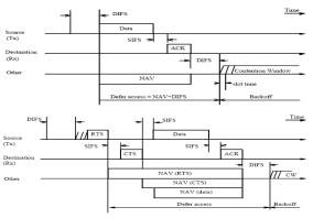
Figure (1): DCF access mechanism: CSMA/CA (up) and RTS/CTS scheme (down)
